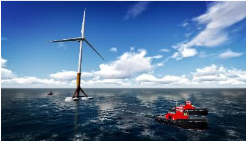
Figure 1. DEMOGRAVI3 towing the wind turbine with foundations
